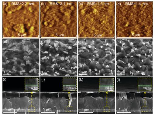
Fig. 3 AFM images of the surface morphology of (a) c-SnO<sub>2</sub>, (b) c(Li)-SnO<sub>2</sub> (c) c-NP-SnO<sub>2</sub> and (d) c(Li)-NP-SnO<sub>2</sub> ETLs. Top and cross-sectional SEM images of perovskite thin films deposited on (e and i) c-SnO<sub>2</sub>, (f and j) c(Li)-SnO<sub>2</sub>, (g and k) c-NP-SnO<sub>2</sub> and (h and l) c(Li)-NP-SnO<sub>2</sub> ETLs.
