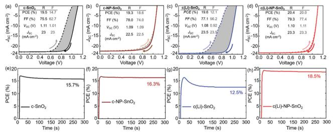
Fig. 2 Reverse (R) and forward (F) J-V scans and stabilized PCE (s-PCE) derived from MPP tracking of champion PSCs with (a and e) c-SnO<sub>2</sub>, (b and f) c-NP-SnO<sub>2</sub>, (c and g) c(Li)-SnO<sub>2</sub> and (d and h) c(Li)-NP-SnO<sub>2</sub> ETLs.
