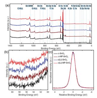
Fig. 4 (a) Survey spectra, (b) Li 1s emission, and (c) Sn 3d<sub>5/2</sub> emission of the four different ETL configurations c-SnO<sub>2</sub>, c-NP-SnO<sub>2</sub>, c(Li)-SnO<sub>2</sub>, and c(Li)-NP-SnO<sub>2</sub> measured by XPS. For shape comparison, the spectra in (c) were normalized and shifted
