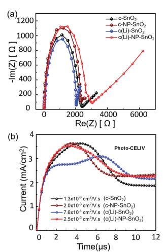
Fig. 6 (a) Electrochemical impedance spectroscopy (EIS) and (b) photogenerated charge extraction by linearly increasing voltage (photo-CELIV) measurements of PSCs with c-SnO<sub>2</sub>, c(Li)-NP-SnO<sub>2</sub> and c(Li)-NP-SnO<sub>2</sub>
