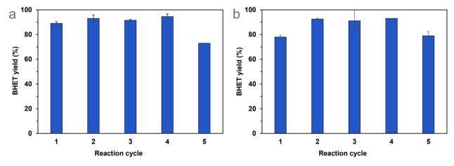
Fig. 7 Catalyst recycling in PET glycolysis applying Si-TEA (a) and Si-TBD (b) catalysts.
