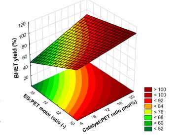
Fig. 5 Response surface plot for the interaction effect between catalyst: PET ratio and EG: PET ratio at a constant temperature of 190  $^{\circ}$ C and with a reaction time of 2 h.
