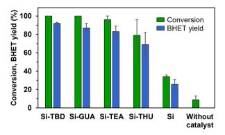
Fig. 3 The catalytic activities of different catalysts in PET glycolysis. Reaction conditions: 190 °C, 10 mol% (or 40 wt% in the case of Si) catalyst (if used), EG: PET ratio of 16, 2 h. BHET yield was determined by HPI C
