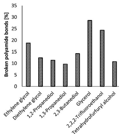
Fig. 4 Effect of the reaction solvent on the ammonolysis of PA66. Conditions: 0.1 M PA66 and 0.1 M benzyl alcohol (internal standard) in solvent (10 mL), 5 mol% La(OTf)<sub>3</sub>, 200 °C, 1 bar NH<sub>3</sub>, 6 h.
