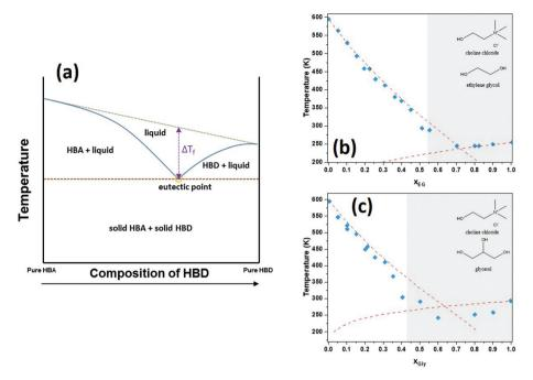
Fig. 2 Representation of solid–liquid phase diagrams for DESs consisting of one HBD and one HBA. (a) General representation; (b) experimental melting points for ChCl: Gly. The gray areas represent the concentration range for which the mixture is liquid at room temperature (*T* = 298.15 K). Data for (b) and (c) were digitized and represented from ref. 38.
