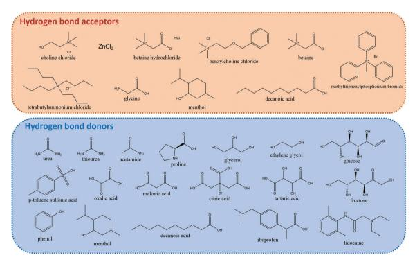
Fig. 3 Some examples of common HBAs and HBDs present in the preparation of DESs.
