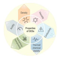
Fig. 4 Important physicochemical properties of DESs for their application in metal recovery.
