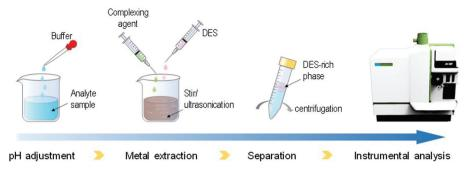
Fig. 13 Schematic procedure of commonly studied DES-based liquid phase metal extraction (LPME method).
