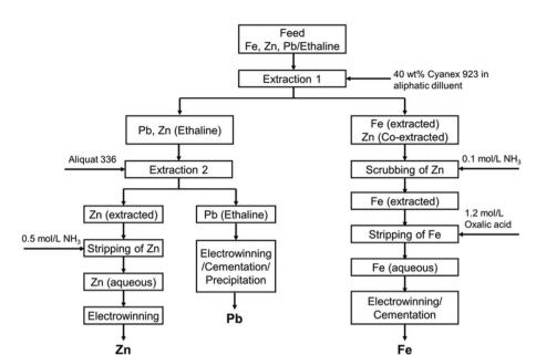
Fig. 16 Proposed flowsheet for the separation and recovery of Fe(III), Pb(III) and Zn(III) a mimicked jarosite waste stream. Reprint with permission from ref. 216, Copyright © 2020, Royal Society of Chemistry.
