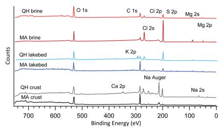
Fig. 2 Broadband photoemission spectra of the six samples measured under vacuum. The photon energy used is 1200 eV. The major peaks are assigned and marked on the plot.
