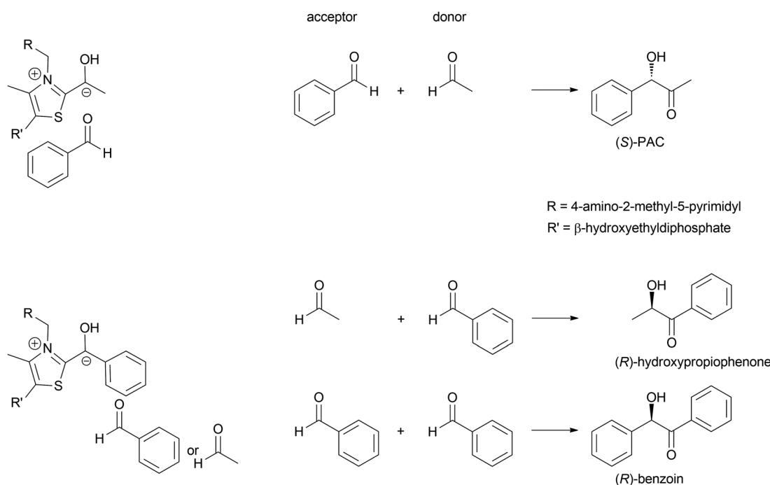
**Scheme 6** Based on the understanding of substrate docking in the active site both the donor pocket and the acceptor pocket can be modulated to accept the desired molecule. In this manner a toolbox of enzymes for all possible combinations could be established.<sup>68</sup>
