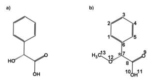
Fig. 1 Schematic structures of (a) mandelic acid (C<sub>8</sub>H<sub>8</sub>O<sub>3</sub>) and (b) alphamethoxy phenylacetic acid (AMPA; C<sub>9</sub>H<sub>10</sub>O<sub>3</sub>). The chiral centre is highlighted with an asterisk.
