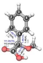
Fig. 7 Comparison of the calculated  $r_e$  (outer semi-transparent structure) and experimentally determined  $r_s$  substitution (black inner spheres) structures of cis-in-perp. The bond lengths and angles for the  $r_s$  structure are shown in black, for  $r_0$  in blue, and for  $r_e$  in gray.
