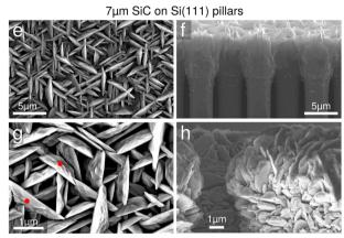
Fig. 2 3C-SiC deposition on Si pillars. (a-d) 5 μm SiC on Si(001) substrate and (e-h) 7 μm SiC on Si(111) substrate. Panels (a, c, e, g) top views; panels (b, d, f, h): side views. Panel (c) is at the same magnification level of Fig. 1(c and e) for direct comparison
