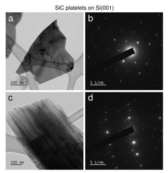
Fig. 4 TEM analysis of thick and thin SiC platelets on Si(001). (a) Brightfield TEM image of a thin SiC platelet on Si(001). (b) Diffraction pattern of the platelet shown in panel a. (c) Bright-field TEM image of a thick SiC platelet on Si(001) with the sample tilted at about 10° with respect to the (111) basal plane. (d) Diffraction pattern of the platelet portion shown in panel (c)
