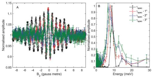
Fig. 3 (A) Oscillation curves measured at different values of incident angle corresponding to specular scattering ( $\gamma_{spec}$ , black),  $\gamma_{spec} - 1^{\circ}$  (red),  $\gamma_{spec} - 2^{\circ}$ (blue) and  $\gamma_{\text{spec}} - 3^{\circ}$  (green) as a function of the integral magnetic field in the second arm of the machine,  $B_2$ .  $B_1$  was fixed at 0 gauss metre. (B) The energy spectra reconstructed from the measurements presented in panel (A).
