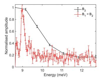
Fig. 6 Comparison of the energy spectra obtained at an incident angle of  $\gamma_{\rm spec}$  + 0.5° when scanning  $B_2$  and holding  $B_1$  at 0 gauss metre (black line), and when scanning along the tilted projection  $B_1 = B_2$  condition (red line). The vertical scale has been truncated to focus on the phonon peak, the elastic peak at 8.6 meV is a delta function (for a 45° tilted projection experiment) and is approx. 500 times more intense than the phonon peak.
