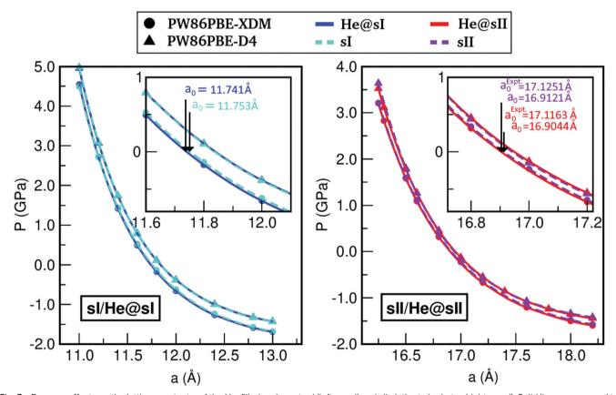
Fig. 3 Pressure effects on the lattice constant a of the He-filled and empty sl (left panel) and sll clathrate hydrates (right panel). Solid lines correspond to the MEOS fits (see Table 1). The zero-pressure lattice parameter values are indicated for the sI/He@sI, while the values at ambient pressure  $(10^{-4} \text{ GPa})$  are reported for the sII/He@sII.
