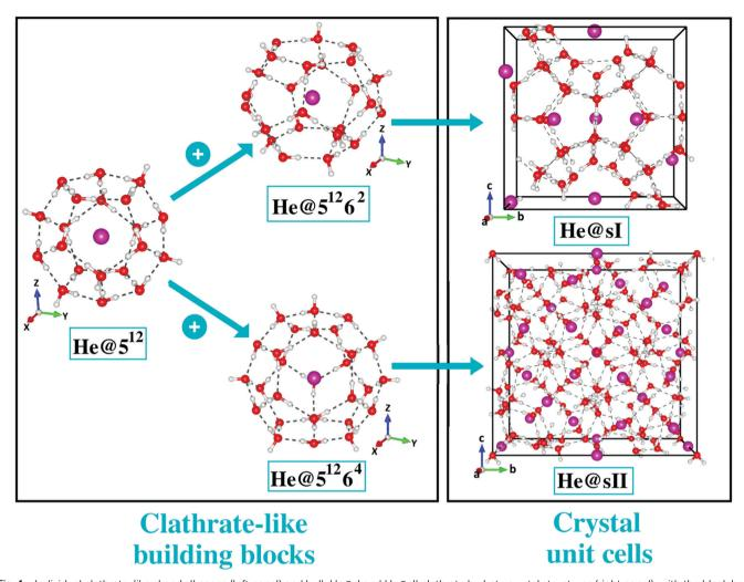
Fig. 1 Individual clathrate-like sl and sll cages (left panel) and bulk He@sl and He@sl clathrate hydrate crystal structures (right panel), with the black box indicating their unit cells. Red color corresponds to oxygen atoms, gray color to hydrogen atoms and magenta color to He atoms.
