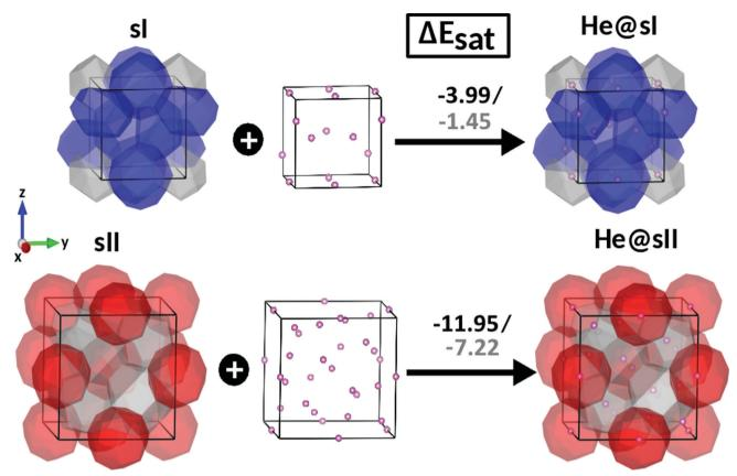
Fig. 5 Saturation energies,  $\Delta E_{\text{sat}}$  in kcal mol<sup>-1</sup>, for fully single cage occupation He@sI and He@sII clathrate hydrates, as computed from the present PW86PBE-XDM/D4 calculations.
