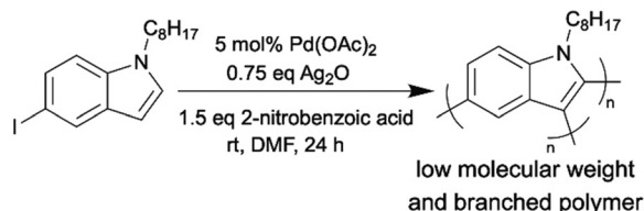
Scheme 10 Room-temperature DARp of 5-iodo-1-octylindole monomer.
