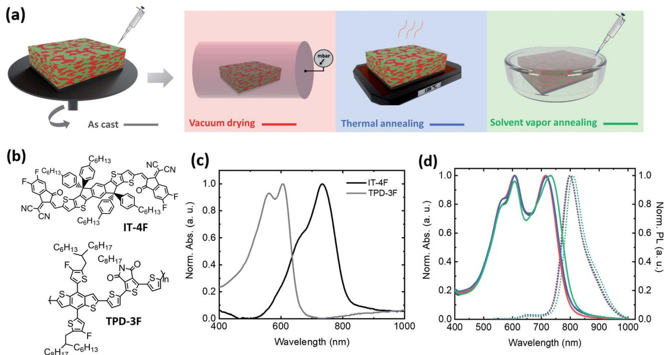
Fig. 1 (a) Schematic representation of the post-processing methods used after spin-casting the BHJ active layer. (b) Molecular structures of small molecule acceptor IT-4F and polymer donor TPD-3F. Normalized UV-Vis absorption spectra of the neat material films (c) and of the blend for each post-processing treatment together with the photoluminescence emission (d). The followed color code is defined in panel (a).
