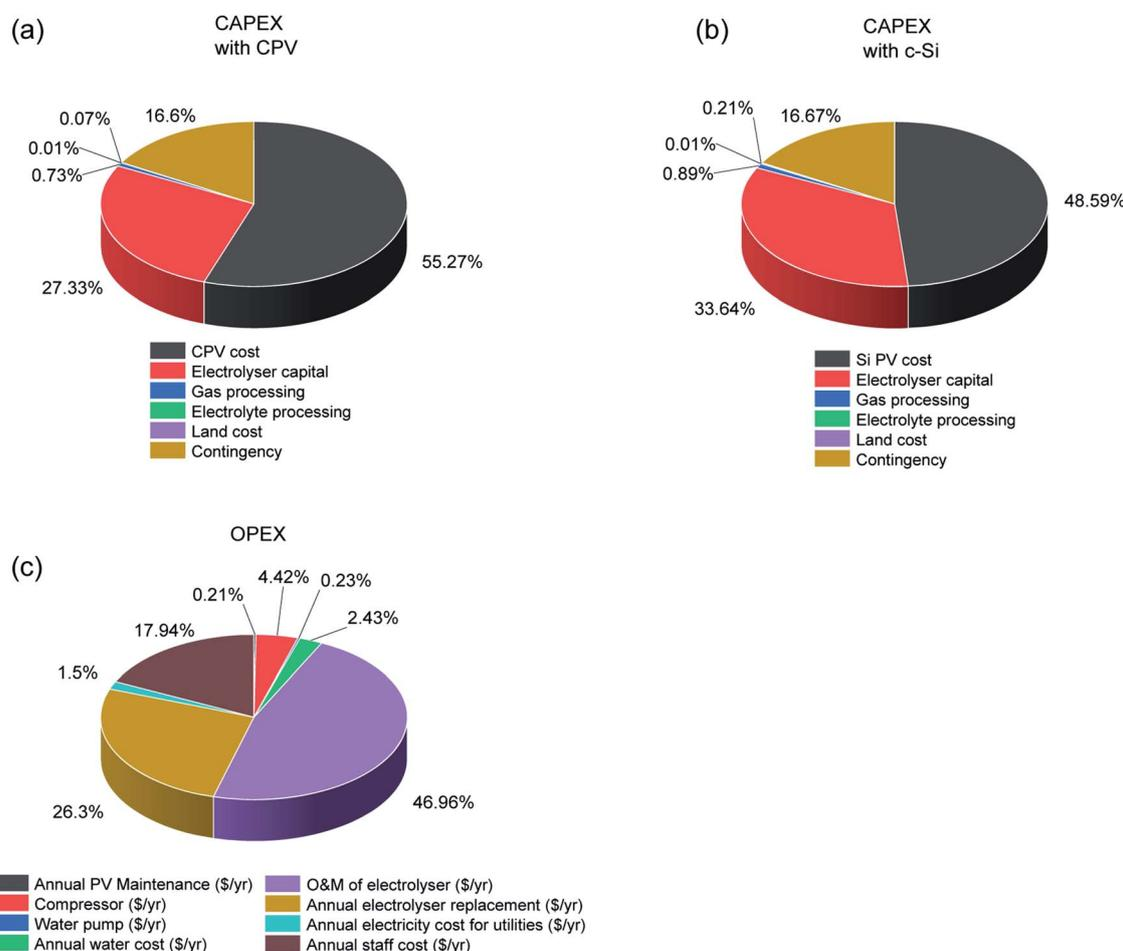
Fig. 3 Breakdown of total capex for a CPV (a) and c-Si PV (b) powered electrolysis process to produce 50 tons  $\text{H}_2$  per day using the assumptions listed in Tables 1 and 2. (c) Annual OPEX for both technologies i.e. CPV-E and c-Si PV-E.
