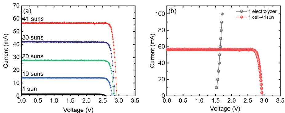
Fig. 1 (a)  $I$ - $V$  characteristics of the InGaP/InGaAs/Ge 3J CPV cell ( $3 \times 3 \text{ mm}^2$ ) from Azur Space under one sun to 41-sun illumination (note the linearity of the current as a function of light concentration). (b)  $I$ - $V$  curve of single alkaline electrolyser (grey) generated using CP measurements overlapped with the  $I$ - $V$  curve of the 3J CPV cell (red) under 41 suns (without the use of Fresnel lenses).
