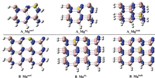
Fig. 2 Top: side view of the **A\_Mg** cluster models doped by replacing one Ga atom of the surface (**A\_Mg<sup>surf</sup>**), first layer (**A\_Mg<sup>FL</sup>**) and bulk (**A\_Mg<sup>bulk</sup>**) with Mg. Bottom: side view of the **B\_Mg** cluster models doped by replacing one Ga atom of the surface (**B\_Mg<sup>surf</sup>**), first layer (**B\_Mg<sup>FL</sup>**) and bulk (**B\_Mg<sup>bulk</sup>**) with Mg.
