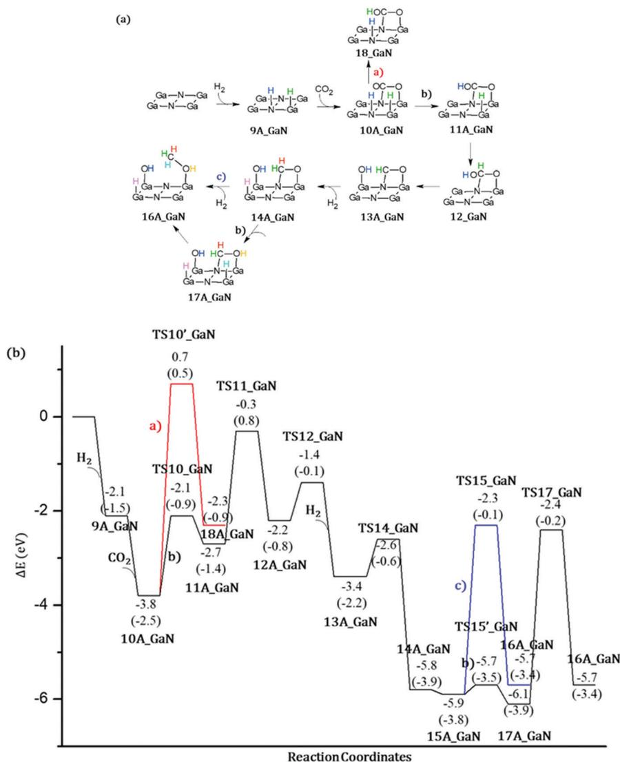
Fig. 6 (a) Schematic representations of all the intercepted stationary points along with the (b) calculated B3LYP energy profile for the  $\text{CO}_2$  conversion to methanol on the  $\text{A}_{\text{GaN}}$  cluster model according to mechanism 2. Energies are in eV and relative to the asymptote of the reactant. Free energies (eV) are shown in parentheses.
