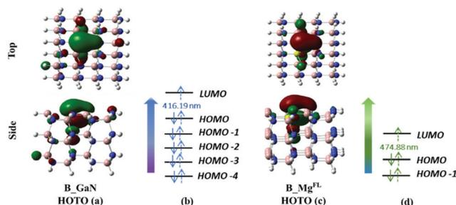
Fig. 4 Top and side view of the HOTO of **B\_GaN** (a) and **B\_Mg<sup>FL</sup>** (c) cluster models; canonical orbitals involved in the transition to the first excited state of **B\_GaN** (b) and **B\_Mg<sup>FL</sup>** (d).
