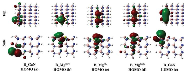
Fig. 3 Top and side view of the HOMO orbitals of **B\_GaN** (a), **B\_Mg<sup>surf</sup>** (b), **B\_Mg<sup>FL</sup>** (c) and **B\_Mg<sup>bulk</sup>** (d); top and side view of the LUMO orbital of the pristine **B\_GaN** (e).
