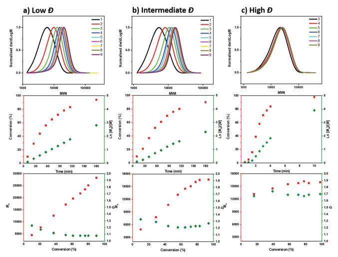
Fig. 2 SEC and kinetic analysis for the synthesis of PMA with different initiators: (a) only EBP, (b)a mixture of EBP: ECP in a ratio 40: 60 and (c) only
