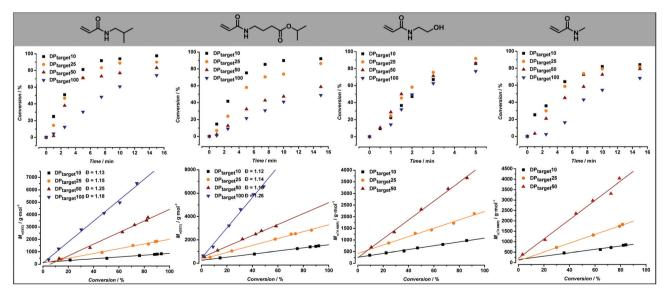
Fig. 4 Summary of the results obtained from the RAFT polymerization screening reactions of four model monomers. Evolution of monomer conversion over time is given for each monomer in the upper panel of the figure. Number-average molecular weight evolution with conversion under variation of [RAFT]/[monomer] ratio is given for each monomer in the lower panel of the figure. The best linear fit of the data points is displayed.
