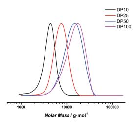
**Fig. 6** SEC traces of poly(1,3-di-boc-guanidinobutyl acrylamide) samples targeting different degrees of polymerization after 8 hours reaction time.
