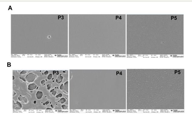
Fig. 8 SEM micrographs of films of copolymers P1-P5 prepared in, (A) chloroform, (B) 2-propanol. Scale bars 200 nm.
