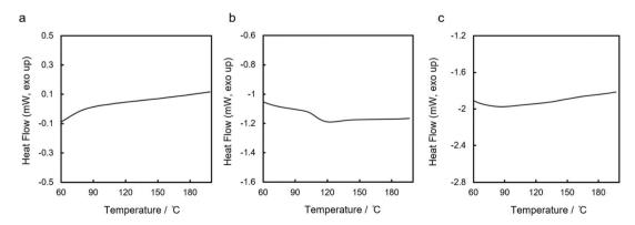
Fig. 4 DSC curves of (a) lin-poly(1,4Si<sub>6</sub>), (b) cyc-poly(1,3Si<sub>6</sub>), and (c) and lin-poly(1,3Si<sub>6</sub>). The second cycle is shown. Heating rate: 3 °C min<sup>-1</sup> for lin-poly(1,4Si<sub>6</sub>), 20 °C min<sup>-1</sup> for cyc-poly(1,3Si<sub>6</sub>) and lin-poly(1,3Si<sub>6</sub>).
