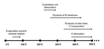
Fig. 6 Proposed polycyclosilane pyrolysis.
