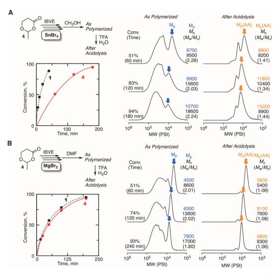
Fig. 5 Comparison between SnBr<sub>4</sub> (A) and MgBr<sub>2</sub> (B) as a catalyst for the ring-expansion cationic polymerization of IBVE with 4: [IBVE]<sub>0</sub>/[4]<sub>0</sub>/[SnBr<sub>4</sub> or  $MgBr_2|_0/[DTBMP]_0 = 380/5.0/5.0$  or 10/0.15 mM in toluene (for  $SnBr_4$ ) or toluene/ $Et_2O$  (90/10 vol%) (for  $MgBr_2$ ) at 0 °C.
