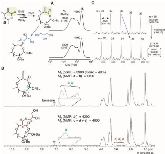
Fig. 6 Ring-expansion cationic polymerization of IBVE with 5 and MgBr<sub>2</sub>, and the post-polymerization reaction of the vinylidene group with thio-glycerol. (A) SEC; (B)  $^1$ H NMR; (C): MALDI-TOF-MS [IBVE]<sub>0</sub>/[5]<sub>0</sub>/[MgBr<sub>2</sub>]<sub>0</sub>/[DTBMP]<sub>0</sub> = 380/5.0/5.0 or 10/0.15 mM in toluene/Et<sub>2</sub>O (90/10 vol%) at 0 °C. The sample was obtained at 49% conversion (1 hour). See the ESI† for the conditions of the post-polymerization reaction.
