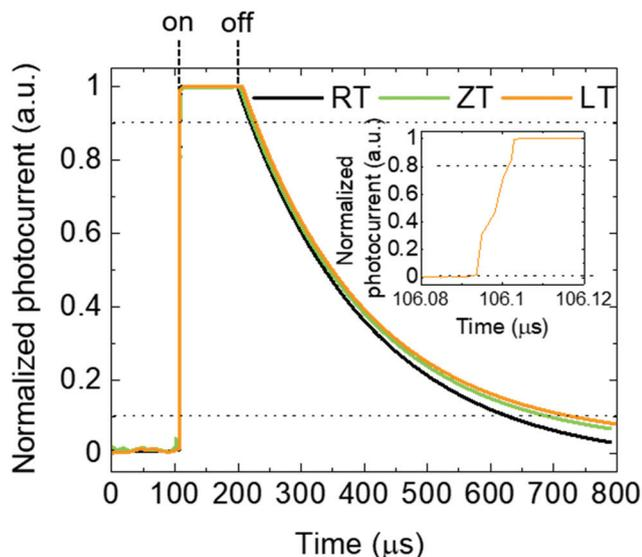
Fig. 7 Response times of MAPbBr<sub>3</sub> single crystals with different dissolution conditions.
