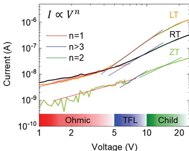
Fig. 4 Dark  $I$ - $V$  characteristics using SCLC method.
