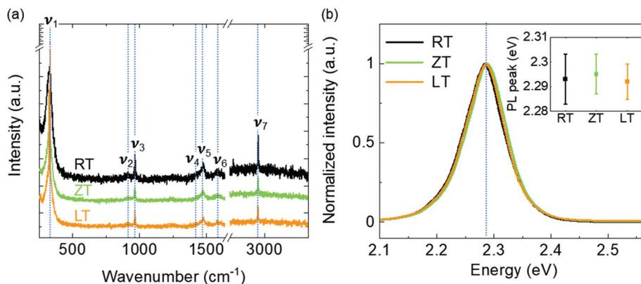
Fig. 3 (a) Raman and (b) PL spectra of MAPbBr<sub>3</sub> single crystal with different dissolved temperatures.
