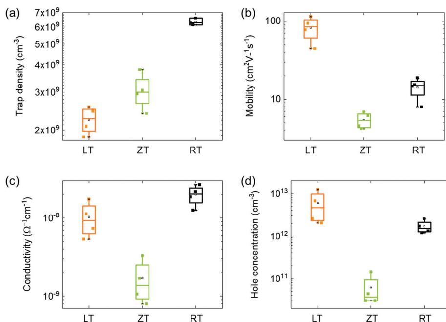
Fig. 5 (a) Trap density, (b) mobility, (c) conductivity, (d) hole concentration of MAPbBr<sub>3</sub> single crystals with different dissolution condition.
