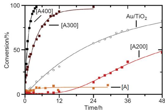
Fig. 6 Kinetic survey of benzyl alcohol dehydrogenation over  $\text{Au}_{25}/\text{SBA-15}$  materials (1.07 wt% Au) as-synthesized [A] (orange) and calcined at 200 °C [A200] (red), 300 °C [A300] (brown), and 400 °C [A400] (black) and comparison data obtained for  $\text{Au}/\text{TiO}_2$  (gray) (reference from the World Gold Council). Reproduced with permission from ref. 212. Copyright 2015 Elsevier.
