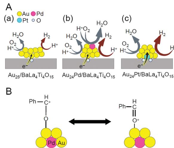
Fig. 38 (A) Proposed structures of  $\text{Au}_{24}\text{M}/\text{BaLa}_4\text{Ti}_4\text{O}_{15}$  for  $\text{M} =$  (a) Au, (b) Pd, and (c) Pt during the water-splitting reaction. (B) Resonance structures of carbocationic intermediate. Reproduced with permission from ref. 211 and ref. 244. Copyright 2016 Wiley-VCH and 2019 American Chemical Society.
