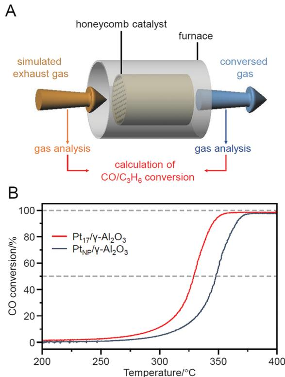
Fig. 22 (A) Schematic of the estimation of CO conversions over Pt<sub>17</sub>/ $\gamma$ -Al<sub>2</sub>O<sub>3</sub> or Pt<sub>NP</sub>/ $\gamma$ -Al<sub>2</sub>O<sub>3</sub> coated on a cordierite honeycomb substrate. (B) CO conversions over Pt<sub>17</sub>/ $\gamma$ -Al<sub>2</sub>O<sub>3</sub> or Pt<sub>NP</sub>/ $\gamma$ -Al<sub>2</sub>O<sub>3</sub>. Reproduced from ref. 235. Copyright 2020 Royal Society of Chemistry.
