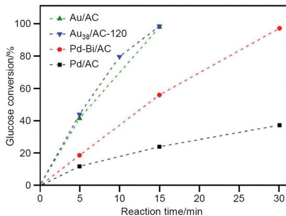
Fig. 7 Glucose conversion vs. time over Pd/AC, Pd-Bi/AC, Au/AC, and Au<sub>38</sub>/AC-120. Reproduced with permission from ref. 213. Copyright 2017 Wiley-VCH.
