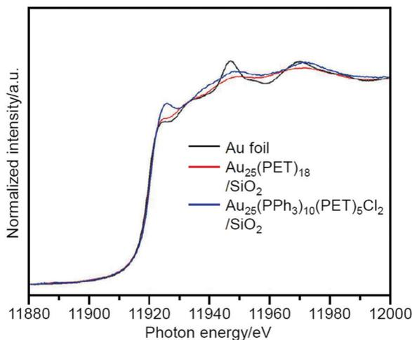
**Fig. 14** Normalized Au L<sub>3</sub>-edge XANES spectra of Au<sub>25</sub>(PET)<sub>18</sub>/SiO<sub>2</sub>, Au<sub>25</sub>(PPh<sub>3</sub>)<sub>10</sub>(PET)<sub>5</sub>Cl<sub>2</sub>/SiO<sub>2</sub>, and Au foil. These spectra indicate that Au in Au<sub>25</sub>(PPh<sub>3</sub>)<sub>10</sub>(PET)<sub>5</sub>Cl<sub>2</sub>/SiO<sub>2</sub> is more cationic than that in Au<sub>25</sub>(PET)<sub>18</sub>/SiO<sub>2</sub>. Reproduced with permission from ref. 222. Copyright 2013 Wiley-VCH.
