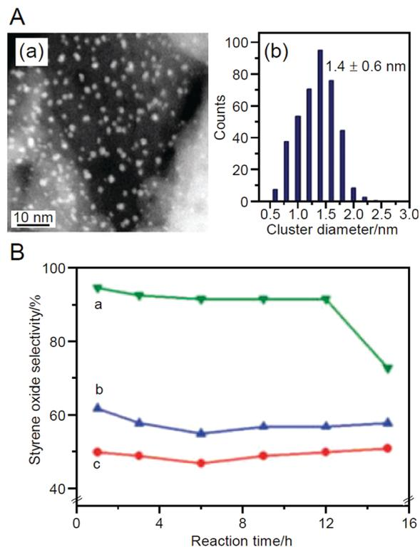
**Fig. 12** (A) (a) Representative HAADF-STEM image of Au<sub>25</sub>/HAP (0.5 wt% Au) and (b) size distribution of the Au NCs. (B) Selectivity of styrene oxide for (a) Au<sub>25</sub>/HAP (0.5 wt% Au), (b) Au<sub>NP</sub>/HAP (0.5 wt% Au) prepared by adsorption of HAuCl<sub>4</sub>, and (c) Au<sub>NP</sub>/HAP (0.5 wt% Au) prepared by impregnation method. Reproduced with permission from ref. 219. Copyright 2010 Royal Society of Chemistry.
