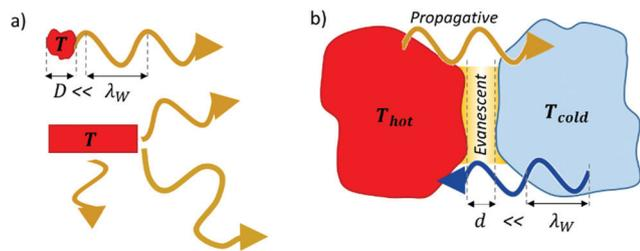
Fig. 1 Nanoscale radiative heat transfer. (a) Sub-wavelength thermal emission from a body at a temperature  $T$  having a size  $D$  smaller than the characteristic wavelength of thermal radiation  $\lambda_W$ . Asymmetric bodies emit also differently along different directions. (b) Near-field radiative heat transfer when the distance  $d$  between two bodies having different temperatures is smaller than  $\lambda_W$ , taking place through evanescent wave tunnelling.
