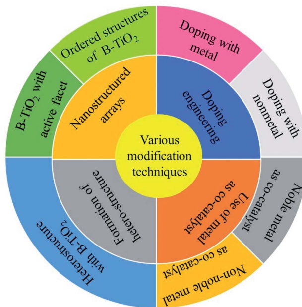
Scheme 2 Schematic diagram shows various modification techniques for B- \text{TiO}_2 to increase the hydrogen generation rate.
