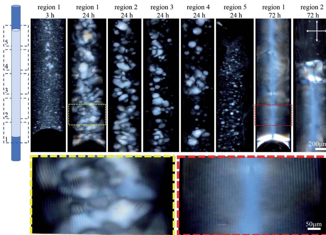
**Fig. 3** Time-series POM images of the 0.4 mm capillary tube filled with 4.5 wt% CNC, and aged vertically as shown in the cartoon. Images were collected along the length of the tube in five regions. Colored dashed boxes show high magnification images. Crossed arrows show the polarizer/analyzer configuration. Rotating the tube around its long axis, and imaging the bottom third shows the lines at different rotation angles implying complete filling of the bottom of the tube (see Fig. S2, ESI†).
