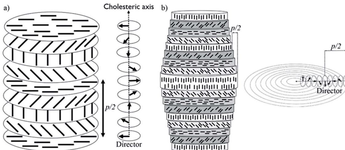
Fig. 1 (a) Planar chiral nematic structure of CNCs and its director field; (b) concentric cylindrical chiral nematic structure of CNCs and its director field. The black rods indicate individual CNCs.
