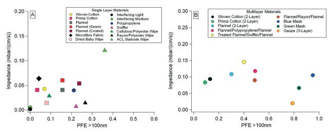
Fig. 6 Plots of impedance vs. PFE (>100 nm) for (A) single layer materials and (B) multilayer material combinations.
