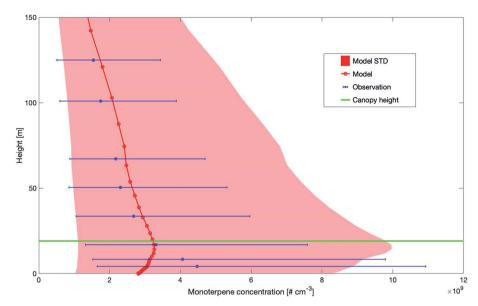
Fig. 3 Vertical profiles of measured and modelled monoterpene median concentrations and ±1 standard deviation (STD) at SMEAR II, Finland for the years 2007-2014 and 2017-2018 (2015-2016 measurement data were not available). The canopy height is marked by a horizontal green line.
