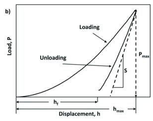
Fig. 1 Schematic of the nanoindentation process and measurement (a) diagram showing the working principles of indenting the sample via loading and unloading, (b) a corresponding load–displacement curve showing the effect of the loading and unloading process. S is the contact stiffness of unloading. Reproduced with permission from Wiley.
