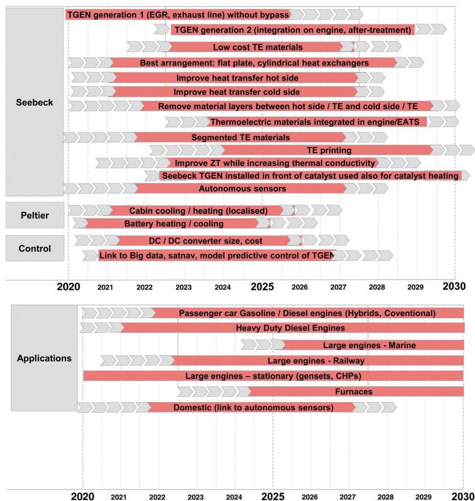
Fig. 10 Roadmap for TEGs and Peltier devices for Automotive sector. (Image courtesy of Ricardo plc.)
