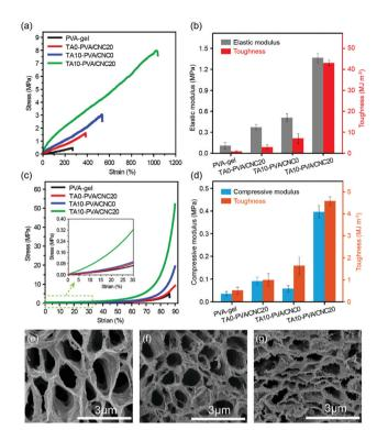
Fig. 3 Typical tensile (a) and compressive (c) stress-strain curves and the corresponding elastic modulus and toughness (b and d) of the PVA-gel, TA0-PVA/CNC20, TA10-PVA/CNC0, and TA10-PVA/CNC20 hydrogels. SEM image of the PVA-gel (e), TA0-PVA/CNC20 (f), and TA10-PVA/ CNC20 (g) hydrogels.
