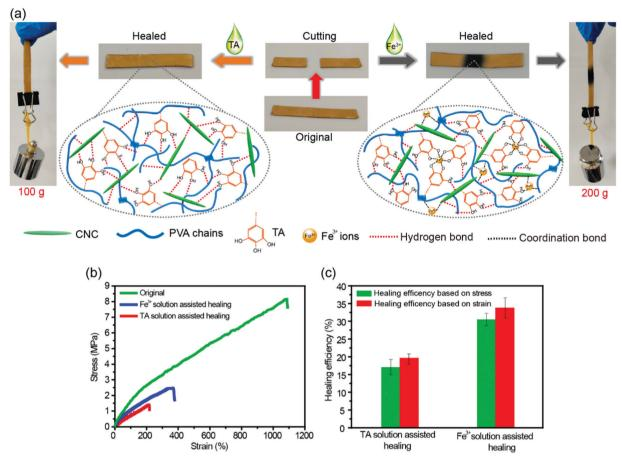
Fig. 6 Demonstration of TA solution (15 wt%) and Fe<sup>3+</sup> solution (0.3 mol L<sup>-1</sup>) assisted healing process of the TA15-PVA/CNC20 hydrogel and its possible mechanism (a). Stress-strain curves of the TA15-PVA/CNC20 hydrogel before and after healing assisted by TA solution (15 wt%) and Fe<sup>3+</sup> solution (0.3 mol L<sup>-1</sup>) (b). Healing efficiency based on fracture stress and strain of the TA15-PVA/CNC20 hydrogel (c).
