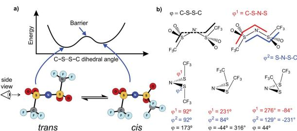
Fig. 1 (a) 1D potential energy surface showing the *cis* and *trans* minima and barrier for interconversion for  $[N(Tf)_2]^-$ . The eye indicates the perspective used in the projection in Fig. 2. (b) Minimum geometries for  $[N(Tf)_2]^-$  and the choice of dihedral angles.
