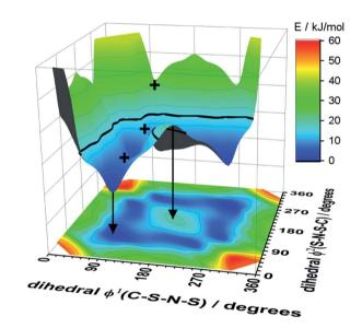
Fig. 4 The upper part of the image is the 3D potential energy surface (PES) of the [N(Tf)<sub>2</sub>]<sup>-</sup> anion and the lower surface the 2D projection. Plus symbols mark selected transition states. The arrows indicate how a local minimum and maximum are mapped on the 2D projection. The bold line at 15 kJ mol<sup>-1</sup> will facilitate comparison with other surfaces. The lowest energy conformer is taken as zero reference.
