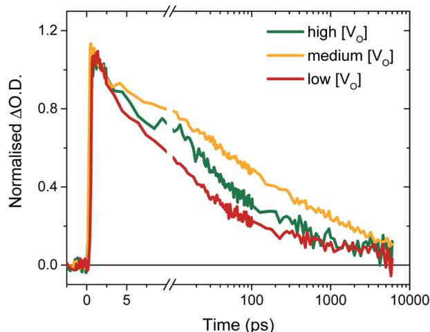
Fig. 5 Normalised ultrafast transient absorption kinetics in 0.1 M  $\text{H}_2\text{SO}_4$ , probing the electron decay at 700 nm from  $\sim 200$  femtoseconds to 6 ns after excitation with 355 nm ( $0.2 \text{ mJ cm}^{-2}$ , no bias) for 'high' to 'medium' and 'low'  $[V_{\text{O}}]$  doping concentrations.
