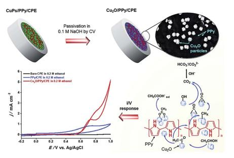
Fig. 14 The preparation of Cu<sub>2</sub>O/PPy/CPE for ethanol electrocatalytic oxidation. Reproduced with permission from ref. 128. Copyright 2020 Elsevier.
