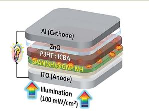
Fig. 11 BHJ PSC with the tool architecture: ITO/SPAN(SH)@GNP(X%) NH/P3HT; ICBA/ZnO/Al. Reproduced with permission from ref. 107. Copyright 2018 Elsevier.
