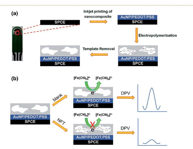
Fig. 3 The electrochemical MIP sensor for NFT determination: (a) the preparation of the electro-synthesized MIP on the nanocomposite modified SPCE. (b) Indirect voltammetric detection of NFT utilizing the  $K_3$ [Fe(CN)<sub>6</sub>]/ $K_4$ [Fe(CN)<sub>6</sub>] as the electrochemical probe. Reproduced with permission from ref. 64. Copyright 2018 Springer.
