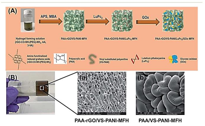
**Fig. 9** (A) The PAA-rGO/VS-PANI/LuPc2/GO<sub>x</sub>-MFH synthesis procedure. (B) SEM images of (a) PAA-rGO/VS-PANI-MFH, and (b) PAA/VS-PANI-MFH. Reproduced with permission from ref. 90. Copyright 2017 Elsevier.
