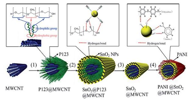
Fig. 12 The preparation of PANI@SnO<sub>2</sub>@MWCNT; steps (1)–(4) represent the dissolution, self-assembly, heating, and *in situ* polymerization. Reproduced with permission from ref. 116. Copyright 2018 Elsevier.
