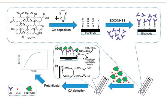
**Fig. 4** Construction of the clenbuterol hydrochloride (CLB) immunosensor. (a) The electrochemical immunosensor format was utilized to detect CLB. (b) The indirect electron transfer for the TMB redox is displayed by the complex TMB/HRP/H<sub>2</sub>O<sub>2</sub> enzyme reaction on the modified SPCE to reduce the creation of the current. Reproduced with permission from ref. 67. Copyright 2018 MDPI.
