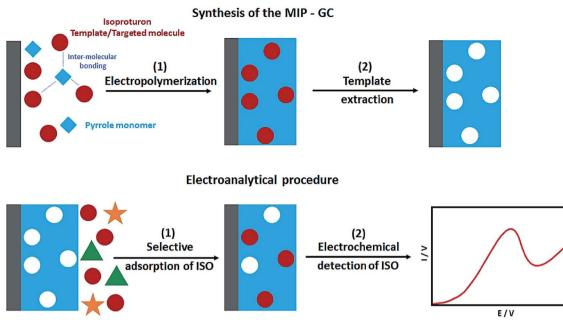
Fig. 8 The process applied to the preparation of the imprinted PPy films on the GC substrate MIPGC and isoproturon electroanalysis. Reproduced with permission from ref. 80. Copyright 2020 Elsevier.
