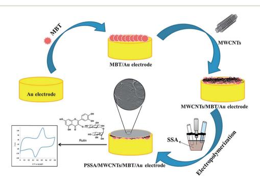
Fig. 5 The preparation process of the PSSA/CNTs/MBT/Au-modified electrode for rutin sensing. Reproduced with permission from ref. 71. Copyright 2018 Elsevier.
