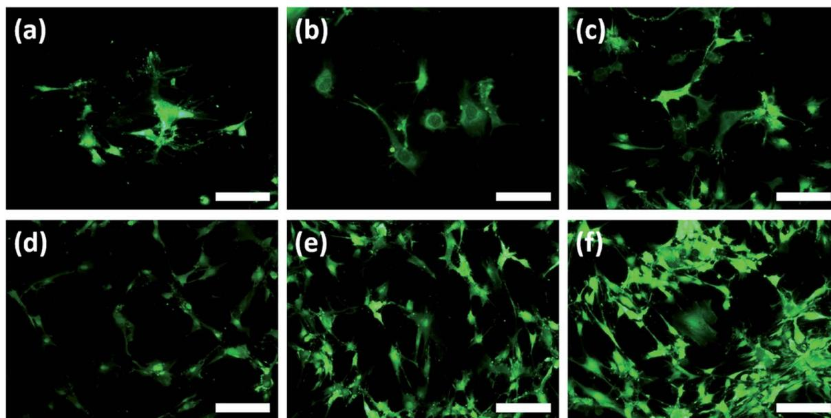
Fig. 4 Fluorescence imaging of HOBs on (a), (d) Ti control, (b), (e)  $\text{TiO}_2$  and (c), (f) flower-like hierarchical Au structures modified  $\text{TiO}_2$  at 12 h and 24 h culturing time (scale bar: 200  $\mu\text{m}$ ) (upper and bottom images represent 12 h and 24 h culturing time, respectively).
