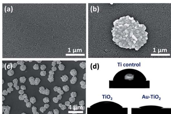
Fig. 2 SEM image of (a)  $\text{TiO}_2$  and flower-like hierarchical Au structures modified  $\text{TiO}_2$  at (b) high and (c) low magnification. (d) Images for contact angle properties of prepared samples.
