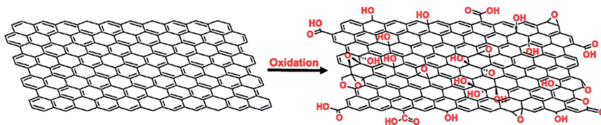
Fig. 2 Oxidation of graphene sheet to form graphene oxide. This figure has been reproduced from ref. 43 with permission from Chem. Rev. , Copyright 2016.
