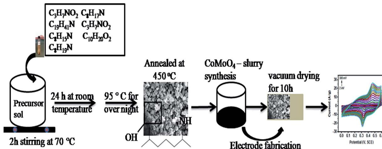
Fig. 1 Schematic diagram of the modified hydrothermal method *via* organic compounds to synthesize CoMoO<sub>4</sub> for fabrication of the electrode.
