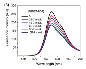
Fig. 4 Fluorescence spectrum of P3HT  $(4.0 \times 10^{-7} \text{ M})$  in chloroform with varying concentrations of the electron acceptor (A) PBDTT-Th and (B) PBDTT-BDT.
