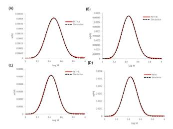
**Fig. 4** Fitting the experimental linear and cyclic mixture with the individual linear and cyclic distributions found by ss and using the LND distributions in Fig. 1 (dashed lines). (A) PSTY-A with targeted  $w_{\rm cyclic}$  = 49.72%, (B) PSTY-B with targeted  $w_{\rm cyclic}$  = 77.96%, (C) PSTY-E with targeted  $w_{\rm cyclic}$  = 95.68%, and (D) PSTY-I with targeted  $w_{\rm cyclic}$  = 99.50%.
