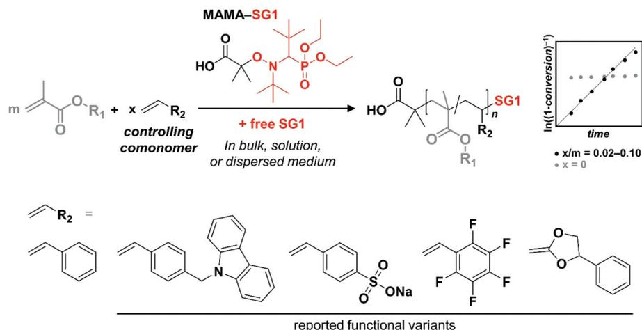
**Scheme 1** The copolymerization approach to achieve control over the SG1-mediated radical polymerization of methacrylates. On the bottom row, besides styrene, the reported *controlling comonomers* providing functionality are presented.
