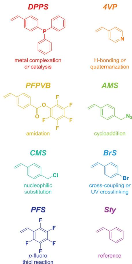
**Scheme 2** Chemical structures, abbreviations, and potential uses of the functionality of the styrenics introduced as *controlling comonomers* in the nitroxide-mediated polymerization of methacrylics in the present contribution.
