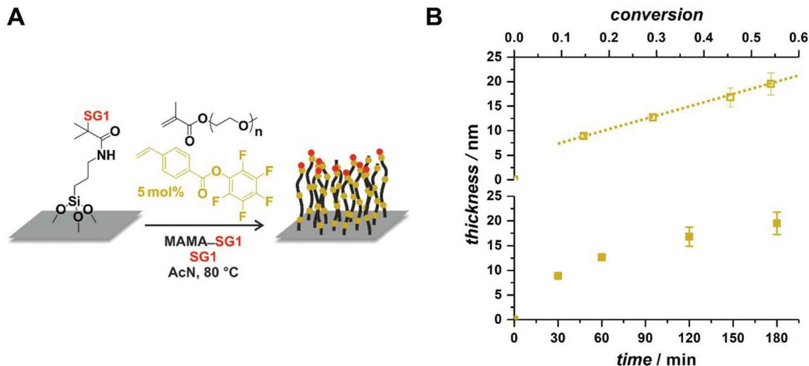
Fig. 8 (A) Schematic depiction of the preparation of POEGMA brushes by NMP on a silicon substrate with the help of PFPVB as *controlling comonomer*. (B) Evolution with polymerization time of the thickness of dry POEGMA brushes obtained by surface-initiated NMP of OEGMA in the presence of 5 mol% of PFPVB as *controlling comonomer* in acetonitrile at 80 °C.
