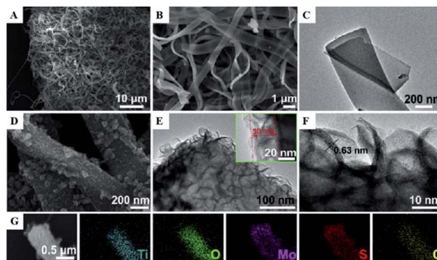
Fig. 11 (A) Low, (B) high-resolution FESEM, and (C) TEM image of  $\text{TiO}_2$  CNBs. (D) FESEM, (E) TEM, and, (F) HRTEM images of  $\text{MoS}_2@ \text{TiO}_2$  CNBs. (G) EDS elemental maps of Ti, O, Mo, S, and C, respectively. Reprinted from ref. 46. Copyright 2017, with permission from Elsevier.
