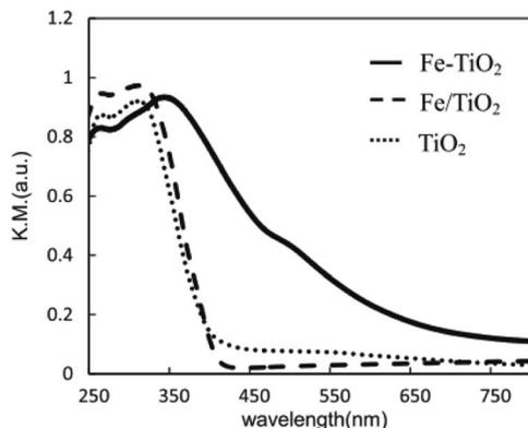
Fig. 6 UV-vis-DR spectra of Fe-TiO<sub>2</sub>, Fe/TiO<sub>2</sub> and TiO<sub>2</sub> photocatalysts. Reprinted from ref. 41. Copyright 2015, with permission from Elsevier.
