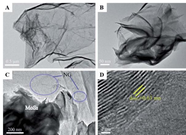
Fig. 8 TEM images of the samples (A–D): (A), N-doped graphene (NG); (B), MoS<sub>2</sub>; (C), MoS<sub>2</sub>/NG; (D) high-resolution image of MoS<sub>2</sub>/NG. Reprinted from ref. 47. Copyright 2020, with permission from Elsevier.
