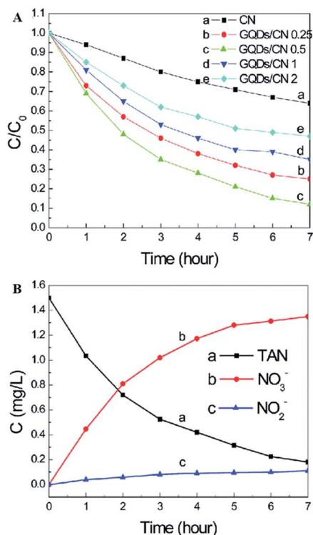
Fig. 10 (A) Effects of the  $g\text{-C}_3\text{N}_4$  and GQDs/CN composite dosage on the photocatalytic treatment of TAN solution. (B) Concentration changes of TAN,  $\text{NO}_2^-$  and  $\text{NO}_3^-$ . Reproduced from ref. 49 with permission from the Royal Society of Chemistry.
