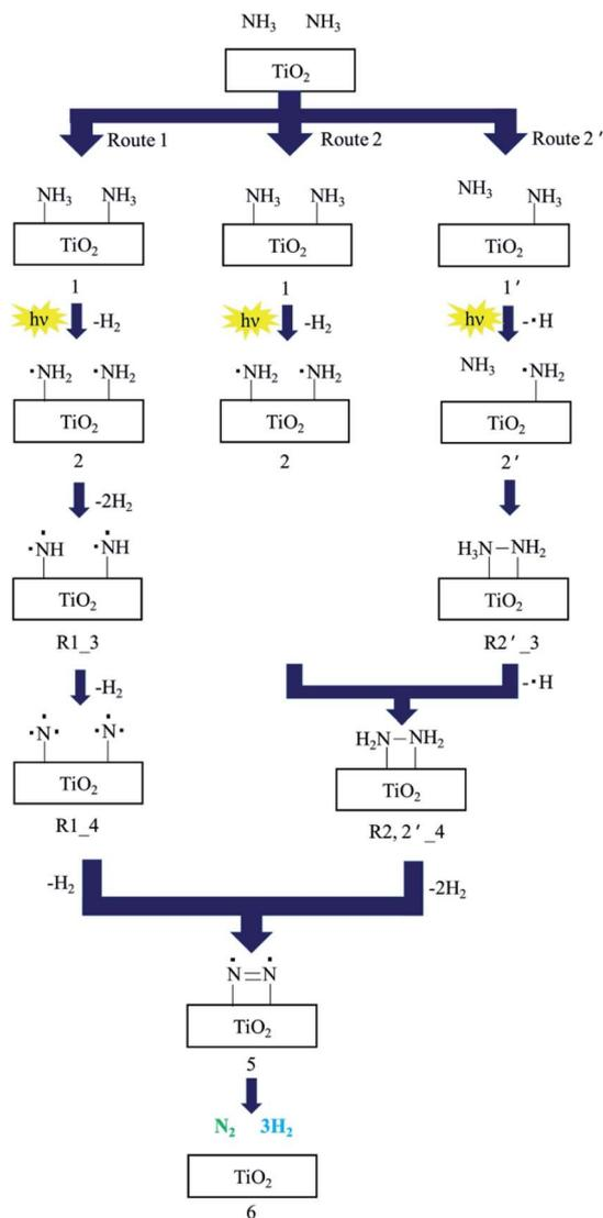
Fig. 4 The suggested reaction mechanism for decomposition of  $\text{NH}_3$  to  $\text{N}_2$  and  $\text{H}_2$  over  $\text{TiO}_2$  photocatalysts. Reprinted from ref. 39, Copyright 2017, with permission from Elsevier.
