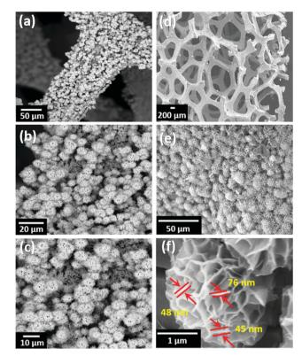
**Fig. 3** FESEM surface morphology of (a-c) MNS, (d-e) MNS-G-2.5 composite, and (f) Enlarged view of the MNS-G-2.5 composite 3D flower.
