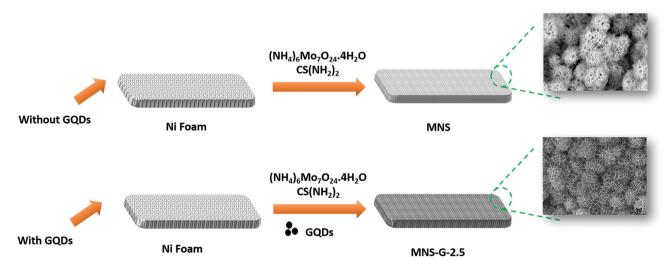
Fig. 1 Schematic illustration of the preparation of MNS and MNS-G-n composites.
