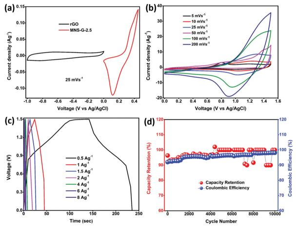
Fig. 7 (a) Cyclic voltammogram curves of rGO and the MNS-G-2.5 composite at a scan rate of 25 mV s<sup>-1</sup>. (b) Cyclic voltammogram curves of the MNS-G-2.5//rGO device at different scan rates. (c) GCD curves of the device at various current densities. (d) Long cyclic performance of the MNS-G-2.5//rGO ASC device at 2 A  $q^{-1}$ .
