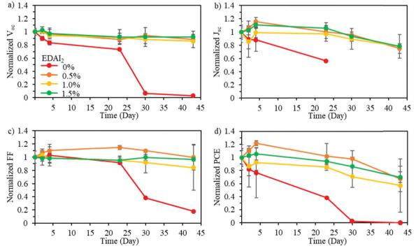
Fig. 6 Normalized (a)  $V_{oc}$ , (b)  $J_{sc}$ , (c) FF, and (d) PCE of the devices containing the active layers of (CsGA)<sub>15</sub> + 0–1.5% EDAI<sub>2</sub> over time in a nitrogen-filled glove box. The (CsGA)<sub>15</sub> + 0% EDAI<sub>2</sub> devices showed a short-circuited behavior after 30 days.
