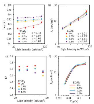
Fig. 5 (a)  $V_{\rm oc}$ . (b)  $J_{\rm sc}$ , and (c) FF as a function of light intensity and (d) photocurrent density as a function of effective voltage for PVSCs with (CsGA)<sub>15</sub> + 0–1.5% EDAl<sub>2</sub>.
