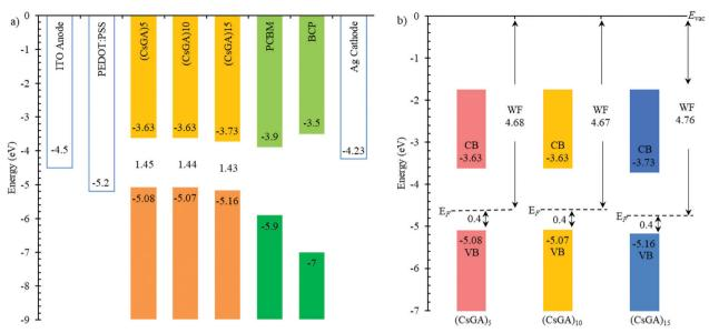
Fig. 4 (a) Band energy diagram of PVSCs with  $(CsGA)_x + 1.5\%$  EDAl<sub>2</sub> active layers, where x = 5, 10 and 15. The band gaps derived from the UV-Vis spectra are indicated. (b) Energy level scheme for the  $(CsGA)_5$ ,  $(CsGA)_{10}$  and  $(CsGA)_{15}$  films with 1.5% EDAl<sub>2</sub> based on the parameters derived from the UPS spectra.
