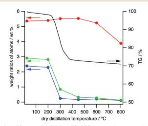
Fig. 3 A TG curve obtained from TG-DSC analysis of a mixture of  ${\bf 1}$  and carbon black (1:1 weight ratio) (black line), and dry distillation temperature-dependent ratios of S (red line), N (blue line) and H (green line) atoms in DDCs determined by elemental analysis. At the point of 25 °C, a mixture of  ${\bf 1}$  and carbon black (1:1 weight ratio) is used, *i.e.*, no dry distillation.
