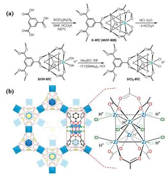
Fig. 6 (a) ZrCl<sub>2</sub>-BTC synthetic scheme beginning with synthesis of Zr-BTC (MOF-808) and (b) proposed structure of ZrCl2-BTC. Reprinted with permission. 41 Copyright 2017 American Chemical Society.
