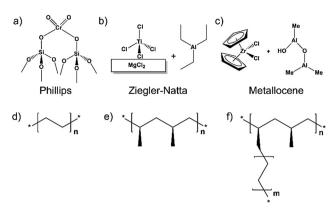
Fig. 1 Structures of (a) Phillips catalyst (proposed), (b) Ziegler-Natta supported catalyst, (c) example metallocene catalyst, (d) linear polyethylene, (e) isotactic polypropylene, and (f) example specialty copolymer of propylene and ethylene.
