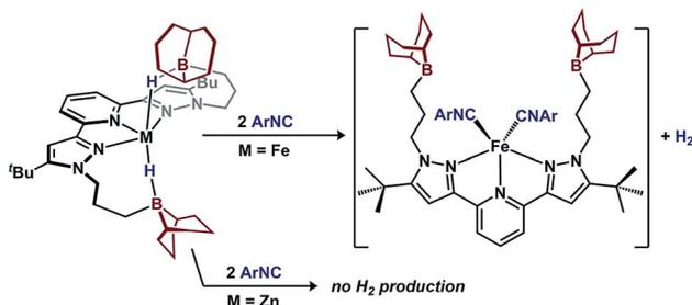
Fig. 6  $\pi$ -acid induced  $\text{H}_2$  extrusion from **1**.
