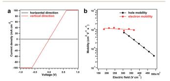
Fig. 5 (a) J-V curves of the 1.6  $\mu$ m-thick COF films measured in the horizontal (black line) and vertical (red line) directions. (b) Dependence of the hole (black line) and electron (red line) mobility in the COF films on the electric field in the vertical direction by a TOF method.
