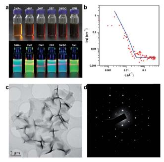
Fig. 3 (a) Photos of the PyVg-COF dissolved in various solvents. Top: concentrated solutions under sunlight; bottom: dilute solutions under 365 nm UV light showing the Tyndall effect. (b) SANS of a DMSO- $d_6$ solution containing concentrated PyVg-COF. The blue line is the curve of a typical 2D planar model. (c) TEM image of a nanosheet of the PyVg-COF at low magnification. (d) SAED of the PyVg-COF nanosheet.
