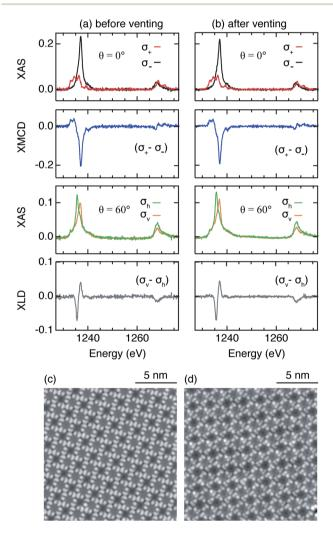
Fig. 4 XAS with circular polarizations, XMCD, XAS with linear polarizations, and XLD measured at the Tb  $\rm M_{4.5}$  edge (a) before and (b) after exposure to ambient conditions for 1 hour (2.3 ML 2H-Pc/Ag(111) + 0.4 ML Tb;  $\mu_0H=100$  mT and 8.0 T for measurements with linear and circular polarizations, respectively, T=6 K). Representative STM images are shown in (c) and (d), respectively (2.7 ML 2H-Pc/Ag(111) + 0.8 ML Tb;  $V_t=-2.0$  V,  $I_t=20$  pA, T=5 K).
