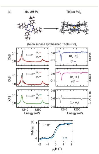
Fig. 5 (a) Schematic of tbu-2H-Pc and Tb(tbu-Pc)<sub>2</sub>. (b) XAS, XMCD, and XLD probed at the Tb M<sub>4.5</sub> edges and (c) magnetization curve probed at the Tb M<sub>5</sub> edge (3.7 ML tbu-2H-Pc/Ag(111) + 0.8 ML Tb;  $\mu_0H=50$  mT and 6.8 T for measurements with linear and circular polarizations, respectively,  $\mu_0\dot{H}=2$  T min<sup>-1</sup> for magnetization curves measurements, T=3 K).
