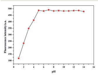
Fig. 6 Effect of pH on the fluorescence intensity of sensor Pyr-Rhy toward  $Ha^{2+}$  in DMSO/ $H_2O$  (1/1, v/v) solution.
