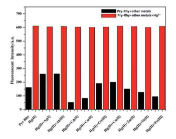
Fig. 7 The black bars represent the fluorescent intensity of sensor Pyr-Rhy and various metal ions (1.0 equiv.) in DMSO/H<sub>2</sub>O (1/1, v/v) solution; the red bars represent the fluorescent intensity of sensor Pyr-Rhy and Hg<sup>2+</sup> (1.0 equiv.) in DMSO/H<sub>2</sub>O (1/1, v/v) solution.
