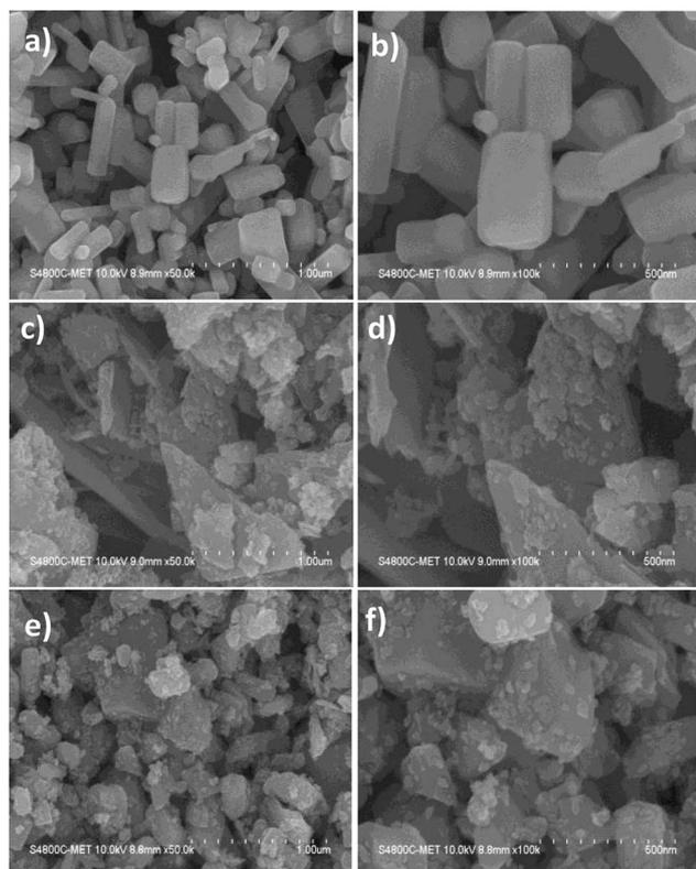
Fig. 3 FESEM images of (a and b) ZnO, (c and d)  $\text{Sn}_3\text{O}_4$ , (e and f)  $\text{ZnO@Sn}_3\text{O}_4$ , respectively.
