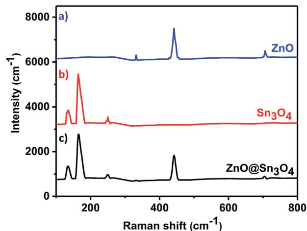
Fig. 2 Room temperature Raman spectra of (a) ZnO, (b) Sn<sub>3</sub>O<sub>4</sub> and (c) ZnO@Sn<sub>3</sub>O<sub>4</sub>.
