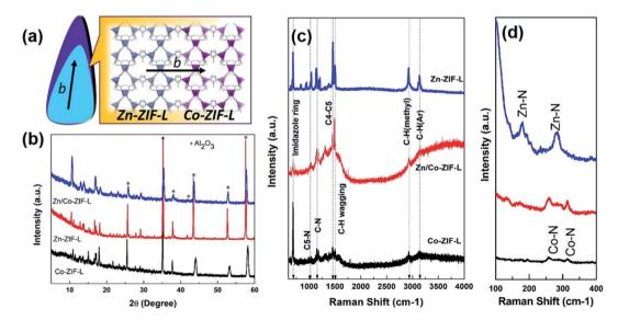
Fig. 3 Structural characterization of ZIF-L membranes. (a) Schematic illustration of the crystal structure for the heterogeneous growth of Co-ZIF-L on Zn-ZIF-L along *b*-axis. (b) XRD patterns of homogeneous membranes (Zn-ZIF-L and Co-ZIF-L) and heterogeneous membranes (Zn-ZIF-L) grown on porous ceramic supports. (c and d) Raman spectra of Zn-ZIF-L, Co-ZIF-L and Zn/Co-ZIF-L samples collected from the corresponding membranes.
