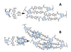
Scheme 1 General illustration of the cross-linking of  $\beta$ -CD with diisocyanate linker (DL) is shown for the binary porous framework polymer (A) and the terpolymer system (B) that incorporates the fluorescent reporter unit (TPE).
