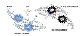
Fig. 3 An illustration of the "on-off" fluorescence quenching mechanism for the FL-PFP/TNP system, where complexes between TPE and TNP at the interstitial sites are likely to induce quenching along with inclusion binding at the CD cavity sites.
